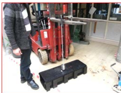
Free fall Impact test EN62262
