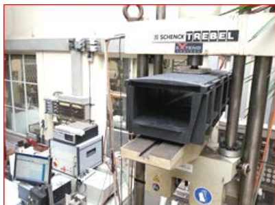
Load test EN124-1 (A15)
